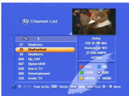
Use the 🔊 buttons to choose your channel, which is then highlighted by a coloured bar. The channel preview appears in the top right-hand corner of the screen. Press 🕏 to confirm your selection. The programme appears on the screen.
